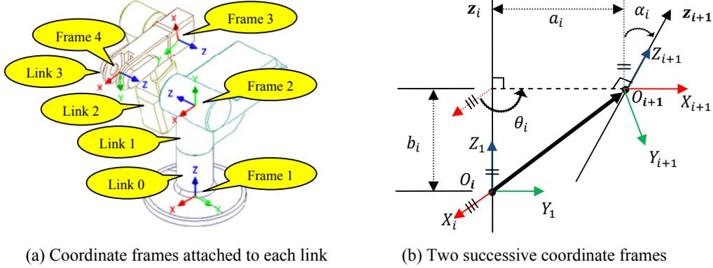
Figure 3: Representation of DH parameters
