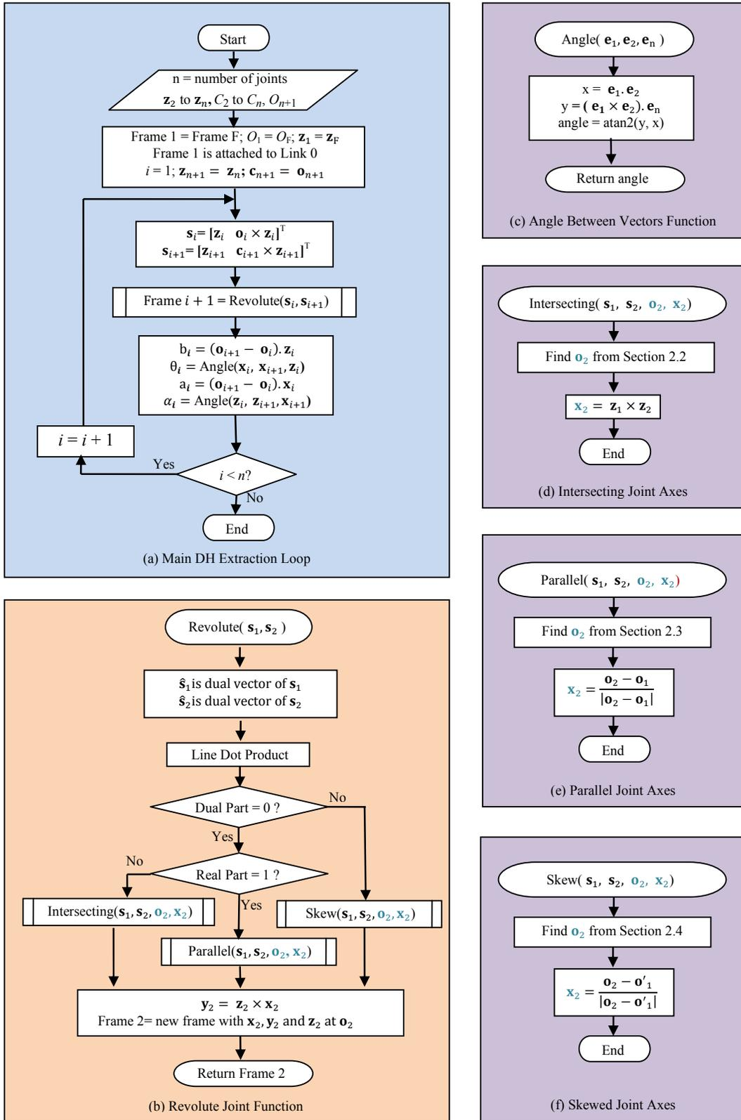
Figure 4: Algorithm for the extraction of DH parameters
