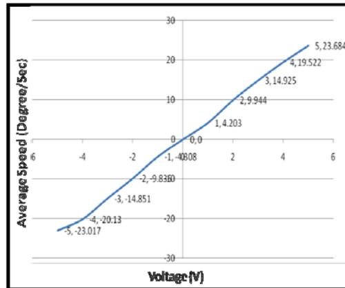
Fig. 7: Calibration of base motor with a person
