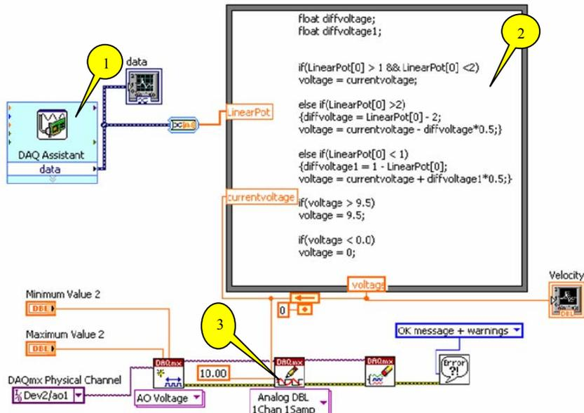
Fig. 10: Block Diagram for treadmill belt control using Cable Potentiometer
