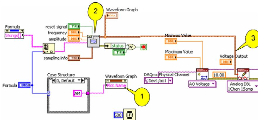
Fig. 3: LabVIEW program for trajectory control
