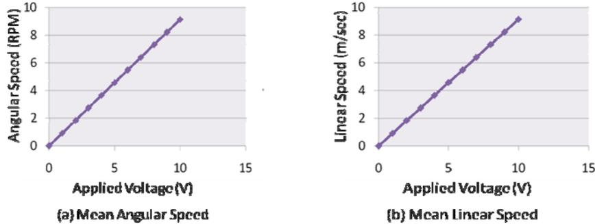
Fig. 5: Calibrated graph for Treadmill belt
