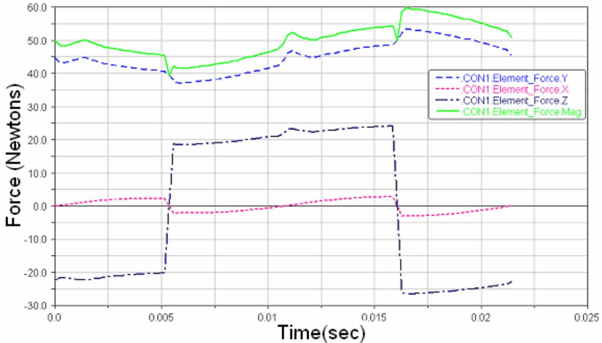
Fig. 13 Contact force between the cutter and comb
