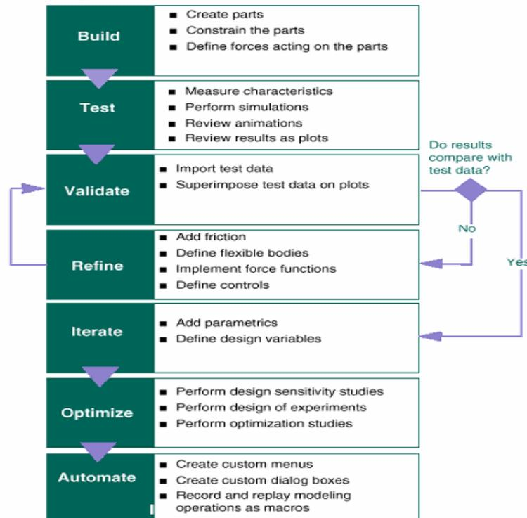
Fig. 3 Flow chart of modeling and simulation in ADAMS
