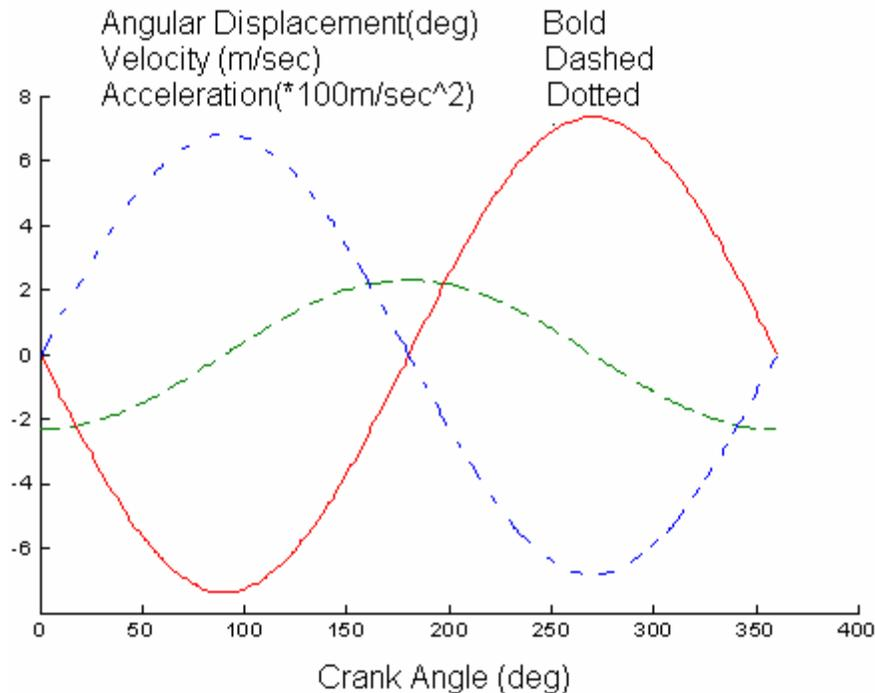
Fig. 17 Fork displacement (deg), velocity (m/s), acceleration (m/s<sup>2</sup>)
