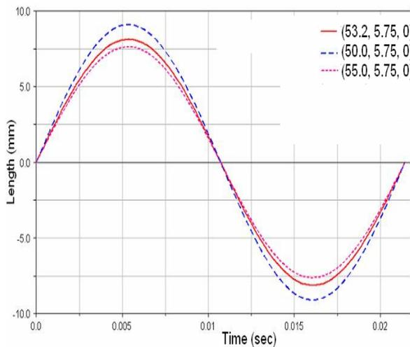
Fig. 9 Z-Displacement of cutter vs. time
