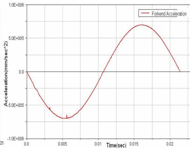
Fig. 15 Fork end Z-acceleration vs. time
