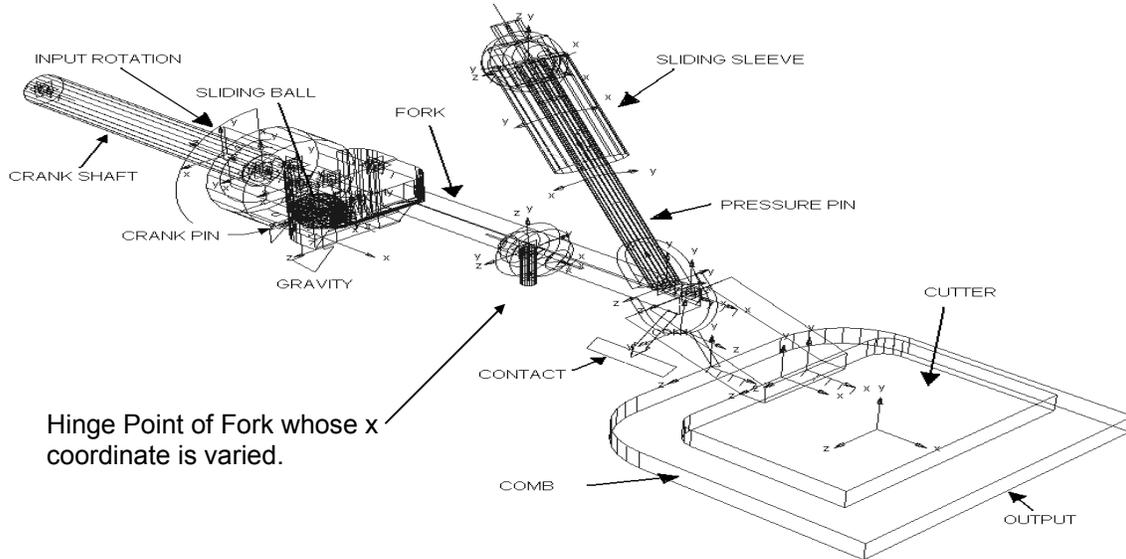
Fig. 2 Different parts in the ADAMS model
