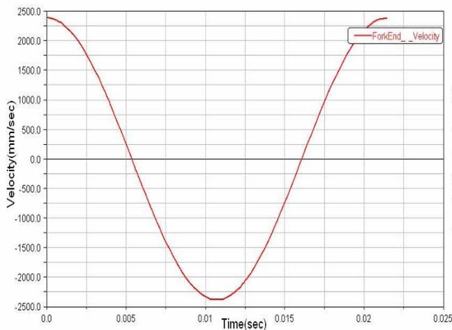
Fig. 14 Fork end Z-velocity vs. time
