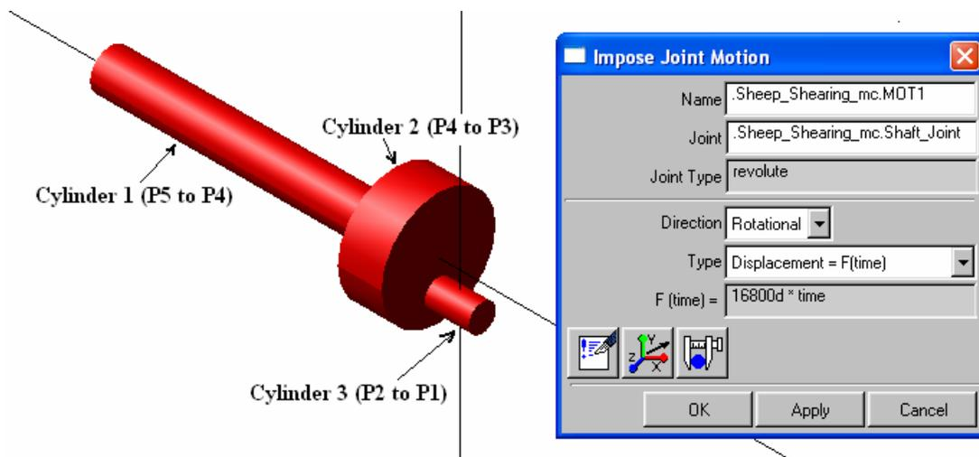
Fig. 5 Shaft with offset pin and input motion specification window
