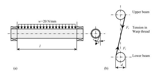
Fig. 3 (a) Warp thread load diagram on beam, (b) Warp thread tension
