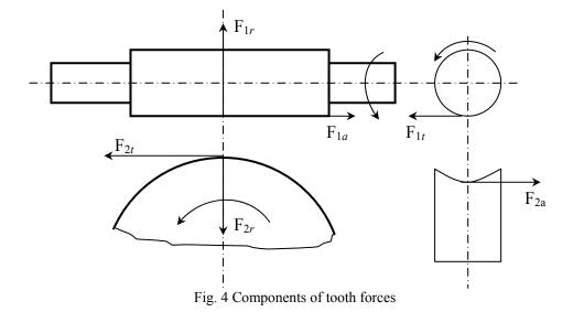
The tangential component on the worm is computed from the input torque as  $F_{1t} = 2T_{in}/d_1$
