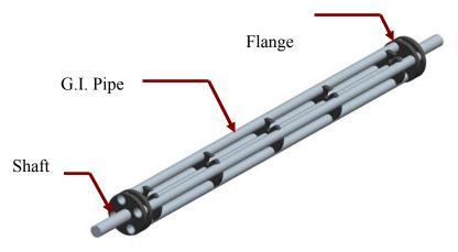
Fig. 5 Disk beam (for Carpet size: 4' X 6')
