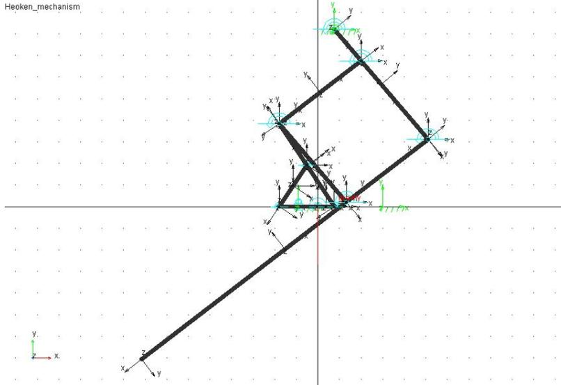
Fig. 7 ADAMS model of the scrapping machine's mechanism
