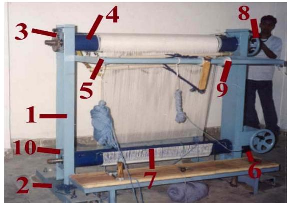
(1. Support Channel; 2. Base Channel; 3. Ratchet and pawl; 4. Upper (Warp) Beam; 5. Shedding Pipe; 6. Tensioning Device; 7. Lower (Cloth) Beam; 8. Handle; 9. Shedding Roller; 10. Bush Bearing)
