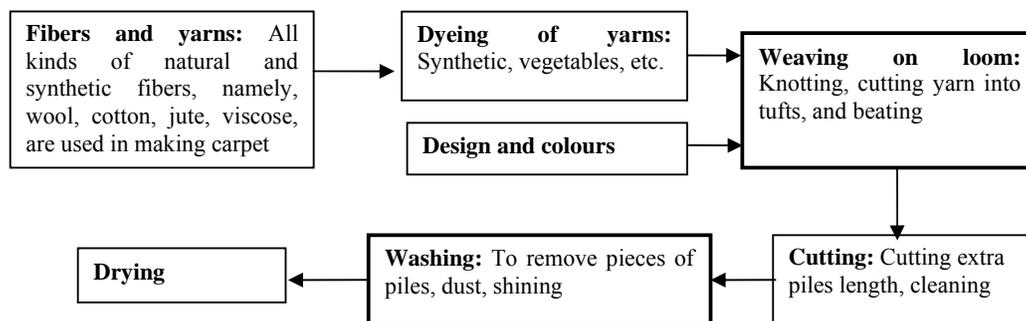
Fig. 1 Flow chart of carpet manufacturing process
