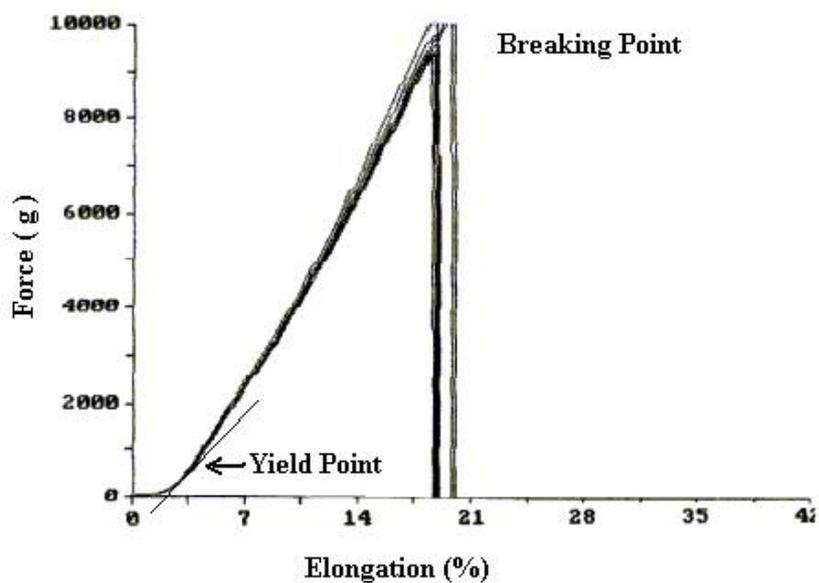
Fig. 2 Tensile test results of warp threads
