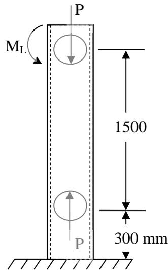
Fig. 6 Schematic diagram of left hand side supports
