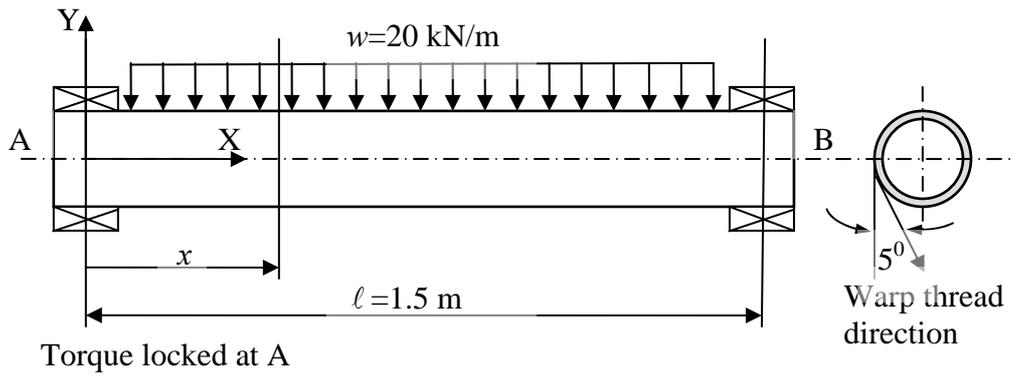
Fig. 3 Load diagram of the upper (warp) beam
