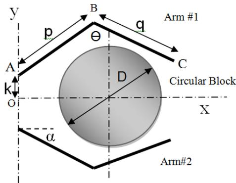
Fig.8: Simplified schematic of the gripper mechanism
