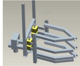
Fig. 4: Solid Model of the gripper
