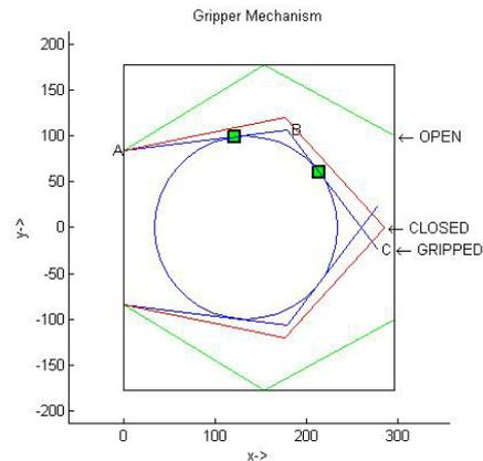
Fig. 9: Screenshot of Matlab screen showing gripper;  $p=180; q=162; k=84; \Theta=120^\circ$
