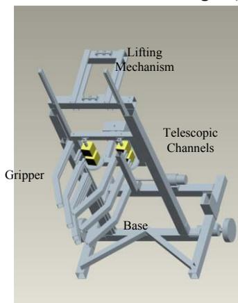
Fig. 3: Solid-model of the robot
