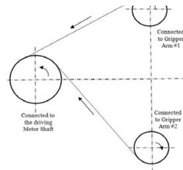
Fig. 5: Three-Pulley arrangement
