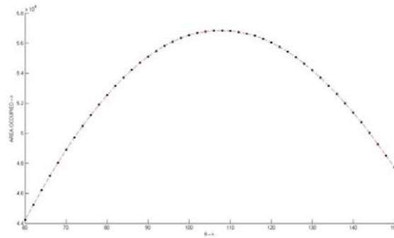
Fig. 10: Graph between the area occupied by the gripper (y axis  $\times 10^{-4} \text{ m}^2$ ) and angle between the two links (x axis deg.)
