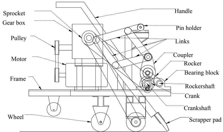
Fig. 5. AUTOCAD assembly drawing of the Carpet Scrapping Machine
