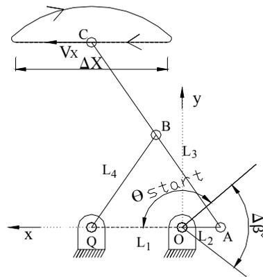
Fig. 3. Proportion of Hoeken's Mechanism
