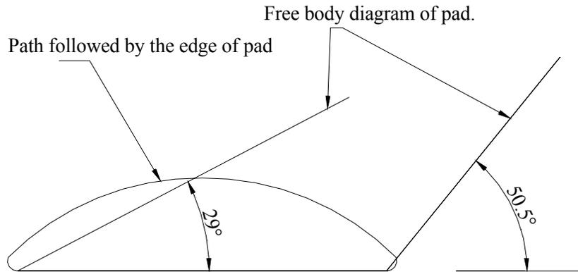
Fig. 2. Scrapper pad path
