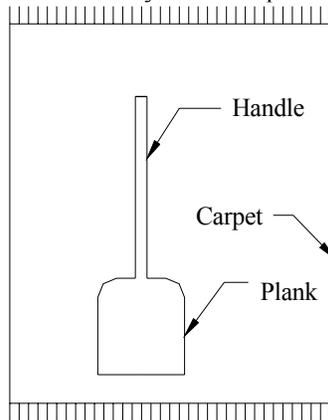
Fig. 1. Existing scrapper pad on carpet
