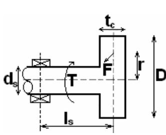
Figure 14: Shaft and Disc
