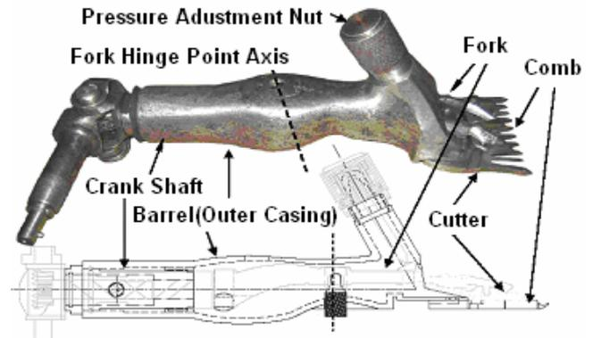
Figure 1: An Existing Sheep Shearing Machine
