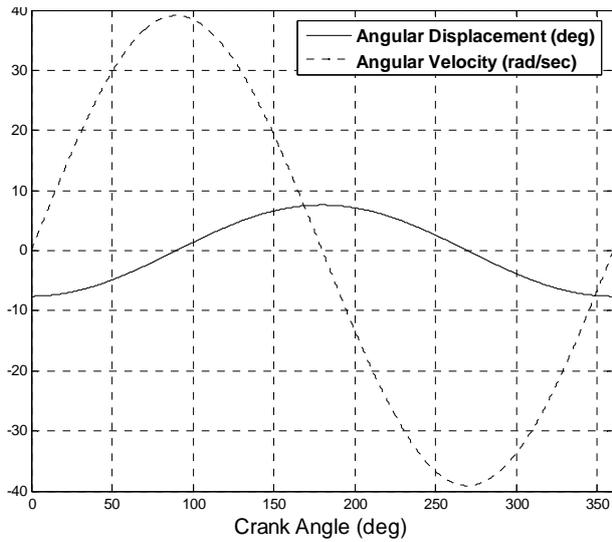
**Figure 19: Output Angular Displacement and Velocity variation against Input Crank Angle**
