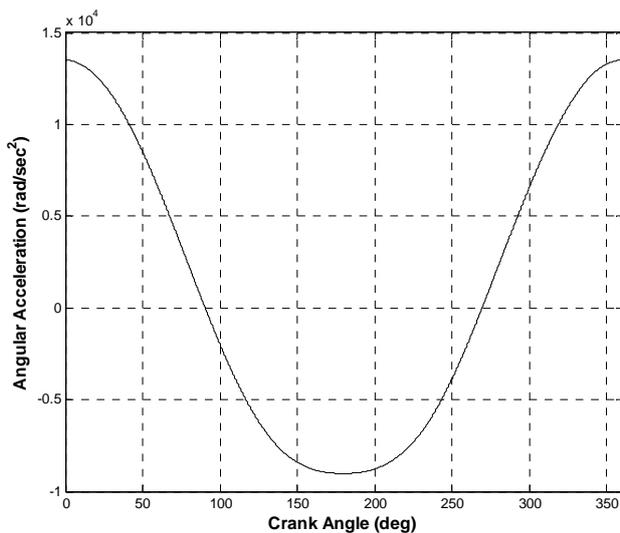
**Figure 20: Output Angular Acceleration Variation**
