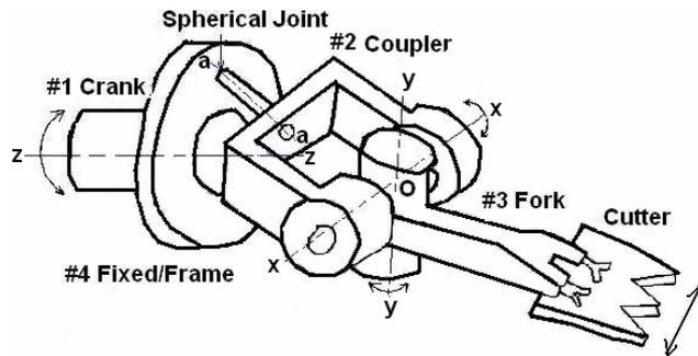
Figure 11: Idea S2-based Sheep Shearing Machine
