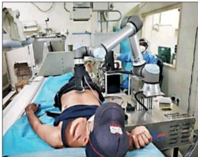
FROM A SAFE DISTANCE: Tele-robotic ultrasound system allows radiologists to manipulate ultrasound probe from a distant location
